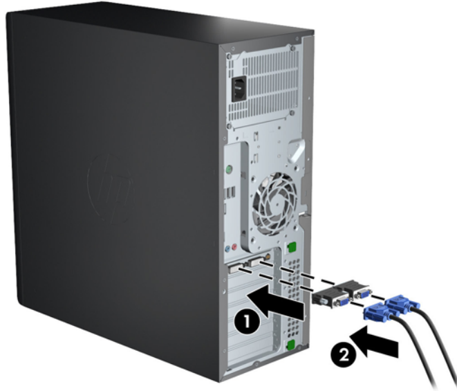
Figure 3-4 Connecting the cables to the workstation
